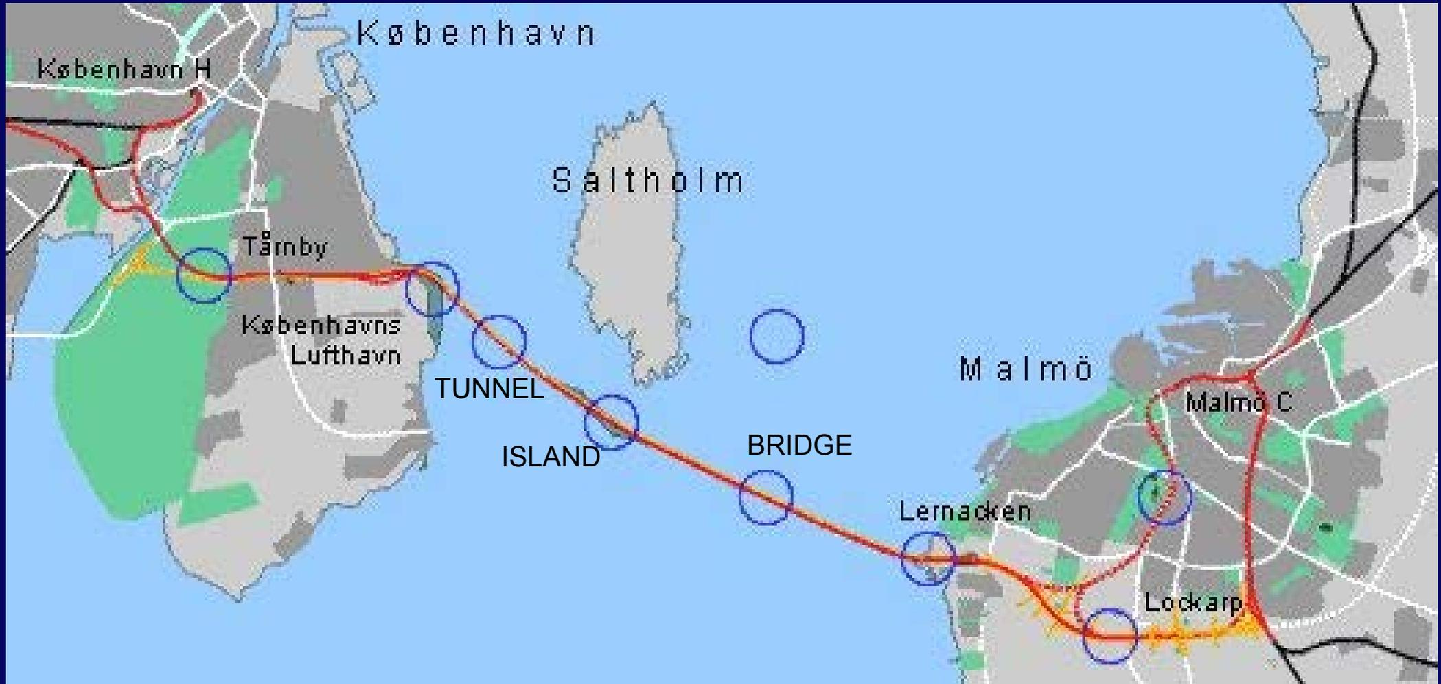
16 KM FIXED LINK: 8 KM BRIDGE, 4 KM ARTIFICIAL ISLAND AND 4 KM TUNNEL
