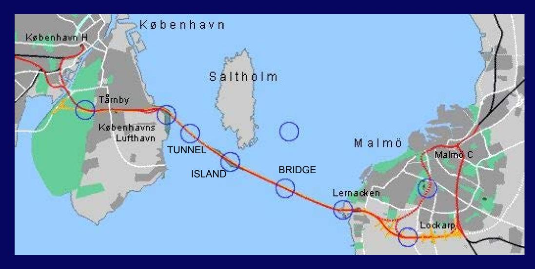
16 KM FIXED LINK: 8 KM BRIDGE, 4 KM ARTIFICIAL ISLAND AND 4 KM TUNNEL
