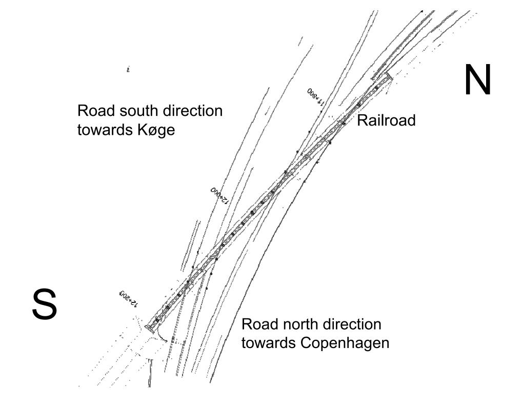
The angle between bridge and road The bridge is 512 m long 15° 20°
