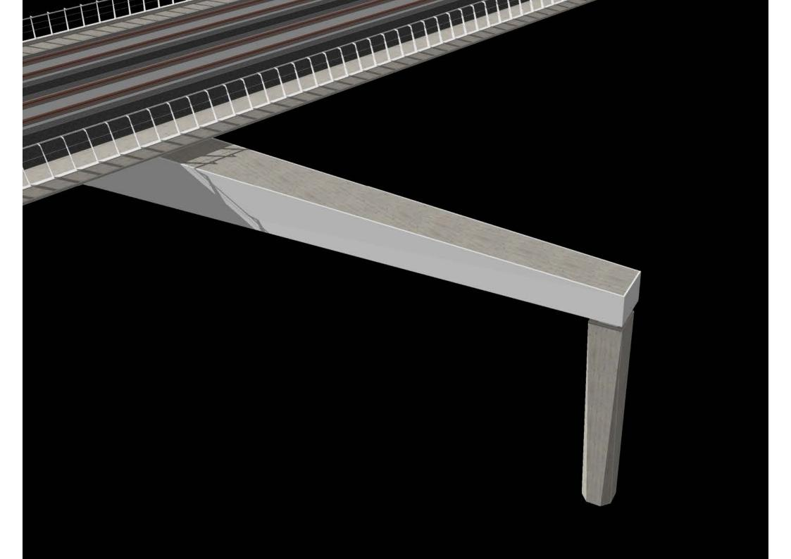
Two bridges anchor point in the middle, expansion joint at both ends
